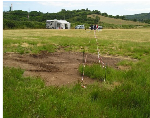
Measurement profile conducted across an individual gas vent within the Latera caldera.
