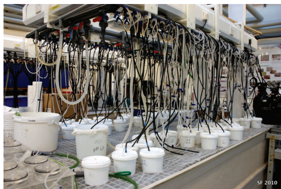
Experimental CO 2 exposure system at the Plymouth Marine Laboratory.
