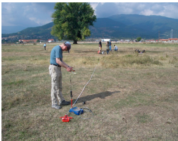
Figure 5 a) Measuring CO 2 content and flux of soil gas across a natural CO 2 vent near Florina, Greece. b) Impact of CO 2 on microbes near Florina, Greece. Numbers of bacteria and archaea were mostly lower at the gas vent but this was reversed by seasonal changes in 2012 at 65–70 cm
