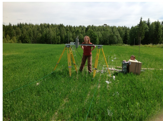
Mapping the reflectance of the crop canopy with an hyperspectral camera
