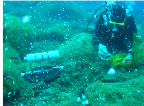
Autonomous probes (developed by the University of Rome) deployed on the sea floor for the continuous monitoring of dissolved CO 2 concentrations.
